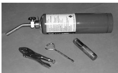
The tools needed for this job are a paint can opener, a hammer, a 3/4 " hole punch, a pair of small vise grips, and a propane torch. The Bulls Eyes I used for this project had one or both beams burned out, so I was not concerned about ruining a rare part.
